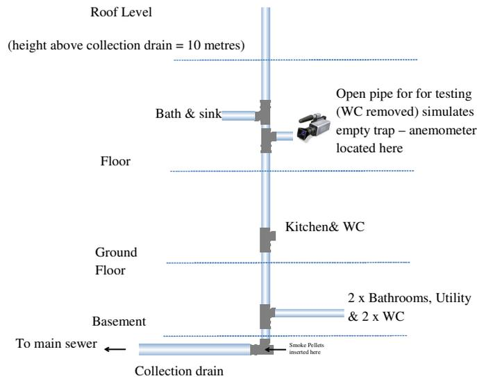
**Figure 1. 3 Storey domestic house used for Airflow measurement and Smoke test**
