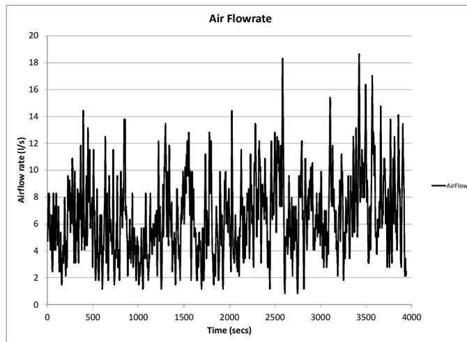
**Figure 3. Airflow recorded in the drainage pipe.**
