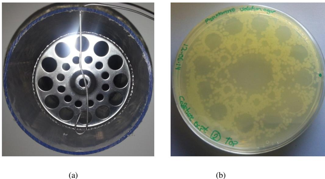
**Figure 4 (a) Passive Pathogen Capture perforated plate (P<sup>4</sup> sampler)**
