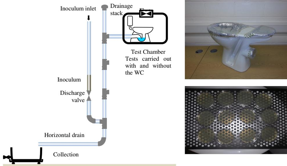
**Figure 2. Laboratory test set-up for model bacteria transfer experiment**
