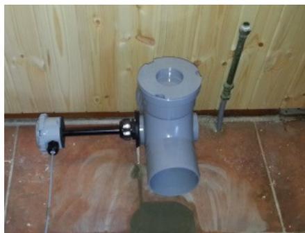
**Plate 1. Installation of the Anemometer to measure airflow velocity and airflow rate**
